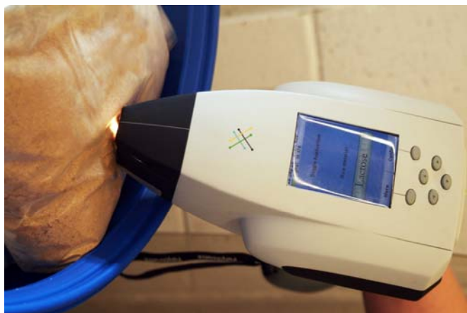
Figure 3. Handheld instrumentation can be brought to the material being identified. Polyethylene liners do not need to be opened for analysis.
